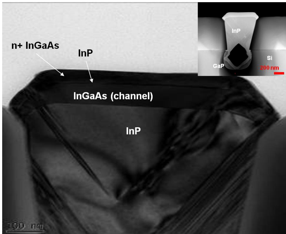
Figure 5- 6. Cross sectional TEM image of InGaAs grown on HT InP template grown at 550 °C. The inset shows the STEM image of the same structure.
