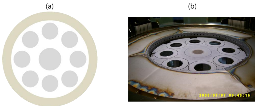
Figure 2-8 (a) Layout of the AIX 2400 G3 susceptor in the 8×3 inch. (b) Photo of the reactor chamber of the AIX 2400 G3 in the 8×3 inch configuration.
