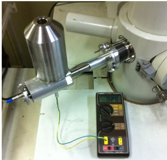
Figure 2.1.7. A photo of the cooling test of the light collectable TEM stage combined with the liquid nitrogen cooling system in a SEM (JEOL, JSM 5200) with a test port.
