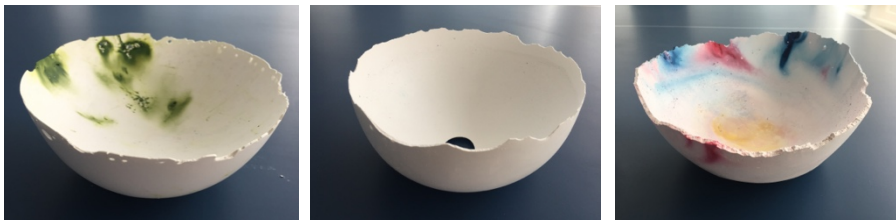
Figure 9. Outputs of Double Blown Balloon Manufacturing Method with and without a Mixture of Watercolors
