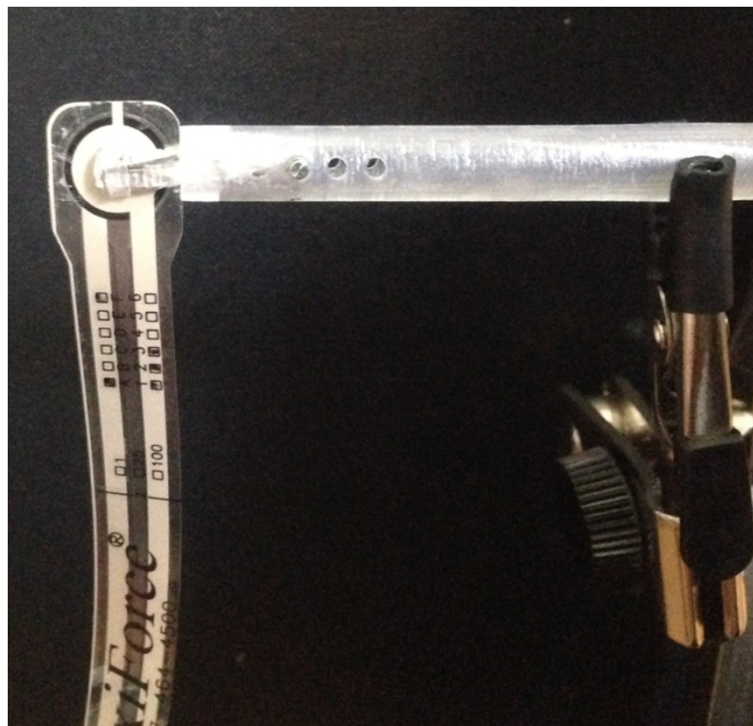
Figure 11 Gripping force measurement experimental setup using Flexiforce.
