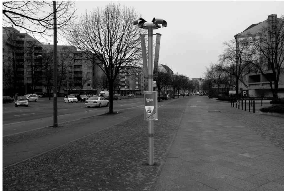
Fig 6. The whole set of i-Give, including the lights and speakers for user-interaction, and bannerhanging facilities for promotion. The inclusive designed handrail at the bottom of the i-Give main body assists wheelchair-users and older people.
