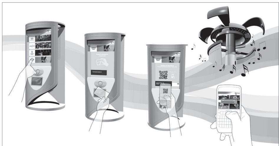
Fig 4. Highly interactive system helps people make donations. Music is presented for promotion and acknowledgement. Commonly used mobile-communication products and applications are adopted for prompting acknowledgement and further promotion of other fundraising activities.
