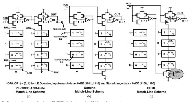
Fig. 7. Examples of range-matching in: (a) PF-CDPD, (b) domino, and (c) PDML match-line structures.
