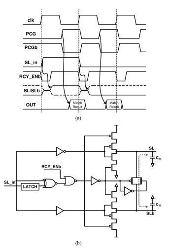
Fig. 11. (a) Timing diagram of the charge-recycling driver and (b) Circuit diagram of the charge-recycling driver.
