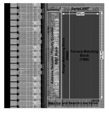
Fig. 12. A  $256 \times 64$ -bit layout of the proposed range-matching TCAM with dynamic match-line RMC and charge recycling-driver.
