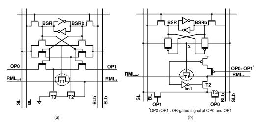
Fig. 6. (a) RMC with a dynamic match-line structure. (b) RMC with a static match-line structure.
