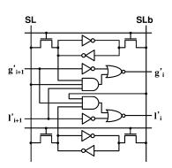
Fig. 5. Range-check cell of an Extended TCAM [9].
