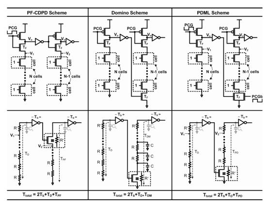
Fig. 9. Match-case evaluation and calculated delays of the PF-CDPD, the Domino, and the PDML schemes.
