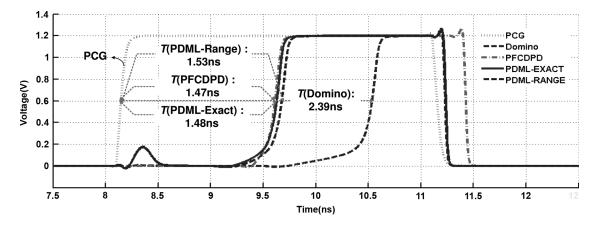
Fig. 10. Post-layout simulated waveform for full exact matching and RM in the worst case.
