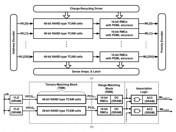
Fig. 2. (a) Block diagram of the range-matching TCAM. (b) 64-bit match-line structure of each entry.
