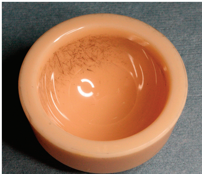
Fig. 2 Photograph demonstrating black discoloration, which is most prominent posterosuperiorly, on the bearing surface of the retrieved alumina liner. No evidence of alumina wear, fracture, or crack formation is evident on gross observation.
