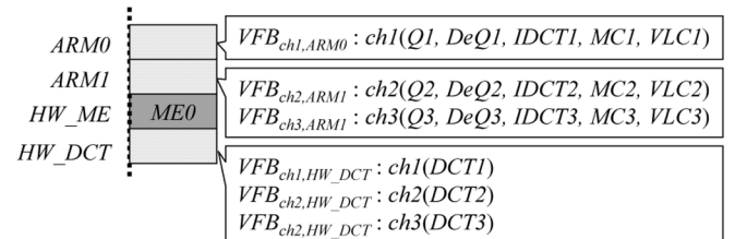
Fig. 6. Function blocks of ch_1 , ch_2 , and ch_3 on ARM_0 , ARM_1 , and HW\_DCT that can be executed simultaneously with ME_0 .
