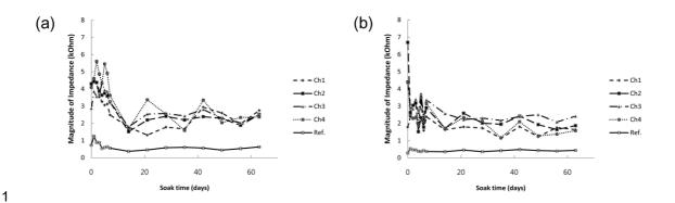
Figure 4. Electrode site impedance monitoring data: (a) magnitude of impedance of Au electrodes on LCP under 37°C PBS soak test, and (b) magnitude of impedance at 75°C.
