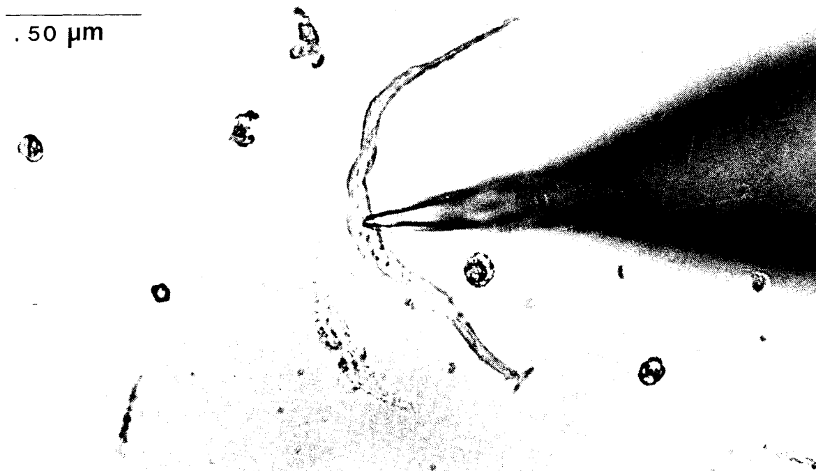
Fig. 2. Light microscopic appearance of a single gastric myocyte obtained from the guinea-pig stomach. A microelectrode tip has been approached to make a giga-seal.
