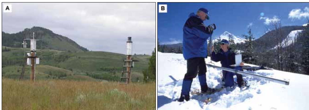
Figure 2 —(A) Examples of shielded (right) and unshielded (left) dual precipitation gauge system used by the USDA Agricultural Research Service, Northwest Watershed Research Center, at the Reynolds Creek Experimental Watershed, Idaho, and (B) snow water equivalent measurement along a snow course transect of the USDA Natural Resources Conservation Service (photo A: Agricultural Research Service; photo B: Ron Nichols, Natural Resources Conservation Service).
