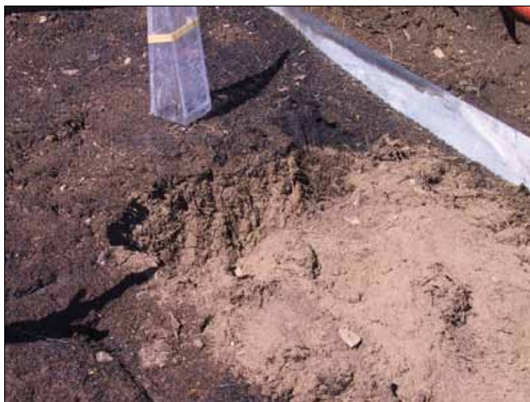
Figure 19 —Dry soil underneath a 2- to 3-cm thick layer of water repellent soil observed immediately after application of 85 mm of rainfall (see Pierson et al. 2008b) over a 1-h period following the Breaks Prescribed Fire, Reynolds Creek Experimental Watershed, Idaho. Soils were strongly water repellent at the mineral soil surface and to a depth of 2 to 3 cm immediately before and after the prescribed fire (photo: USDA Agricultural Research Service, Northwest Watershed Research Center).
