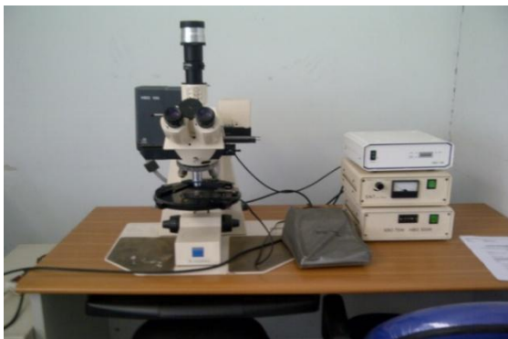
Fig 2. Carl Zeiss Microscope and Point Counter Model F with 500 x magnification
