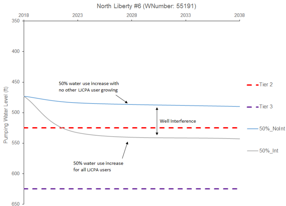
Figure AC-35: Well interference at North Liberty #6 with 50% growth in the LJCPC (North Liberty #7 used as an ASR well)
