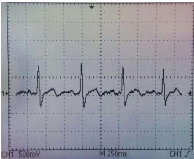
Figure 6: ECG experimentally observed on the oscilloscope by the students.
