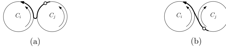
Figure 2.11: Path (bold stroke) traveled by a robot (hollow point) when it passes from a trajectory to another. (a) Both trajectories have the same direction. (b) The trajectories have opposite directions.
