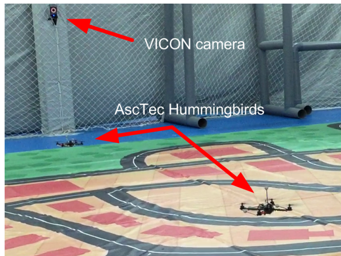
Figure 2.13: Photograph of the indoor testbed used for the preliminary experiments and the aerial vehicles involved.
