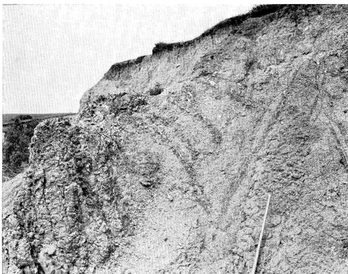
FIG. 2.—Section No. 1 (Norfolk—North Gravel Pit Section). This is a close-up of the central portion of Figure 1. The weathered zones in the Kansan till extend to the base and are about four to five inches wide.
