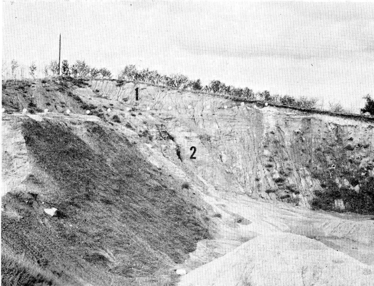
FIG. 5.—Section No. 6 (Einung Gravel Pit). A film of till and loess obscures the true sandy lithology of the lower bed at the east end of this pit. The dotted line follows the contact of the Kansan till (1) and distorted zone between the till and underlying Early Kansan gravel (2).
