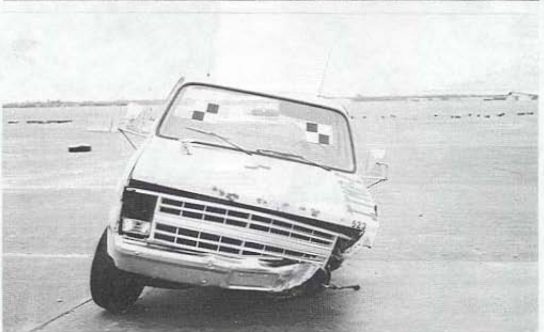
Figure 31. Vehicle Damage, Test ITMP-2
