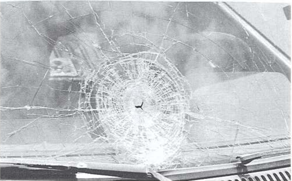
Figure 17. Vehicle and Windshield Damage, Test I-1
