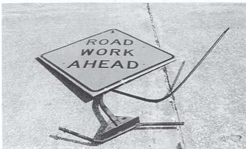
Figure 15. System No. 1 Damage, Test I-1
