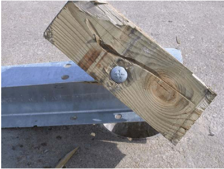
Figure 4. System Damage, Bogie Test WB-1
