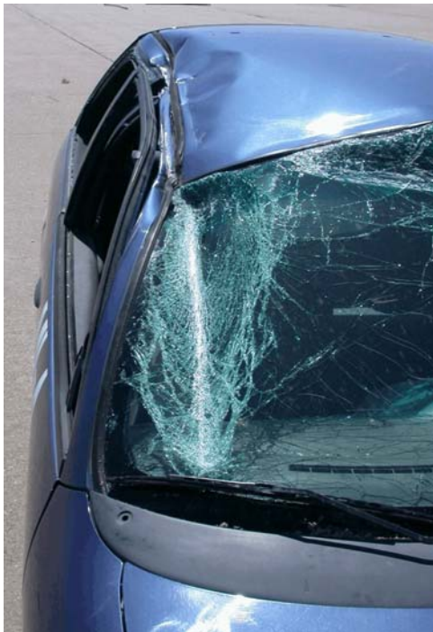
Figure 25. Windshield and Roof Damage, Test MI-4
