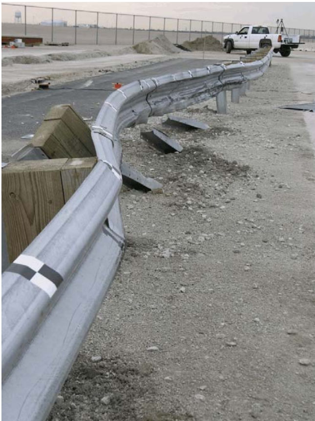
Figure 23. Midwest Guardrail System Barrier Damage, Test 2214MG-2
