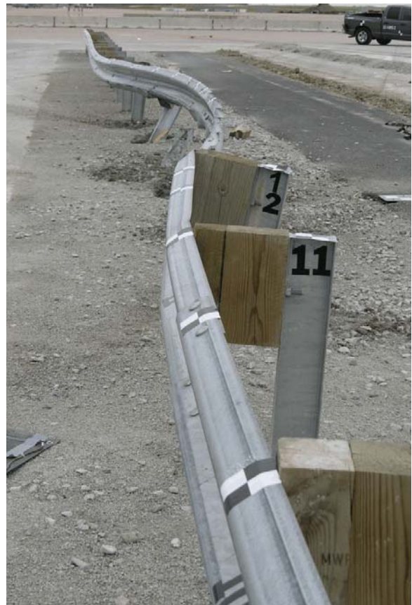
Figure 23. Midwest Guardrail System Barrier Damage, Test 2214MG-2
