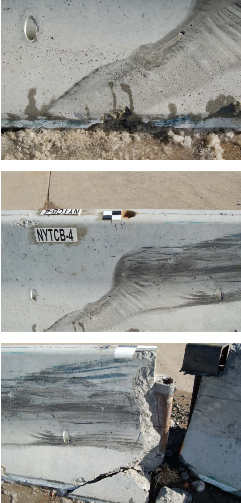
Figure 26. Barrier No. 4 Damage, Test NYTCB-4
