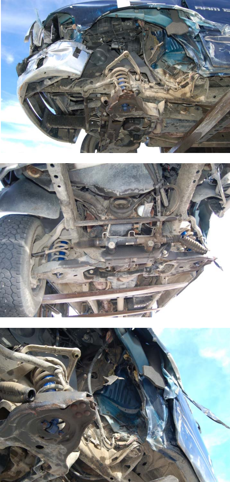
Figure 36. Undercarriage Damage, Test NYTCB-4
