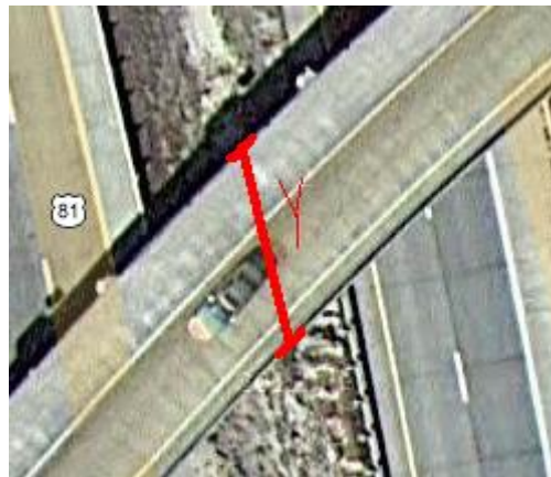
Figure 4. Measurement of Bridge Width
