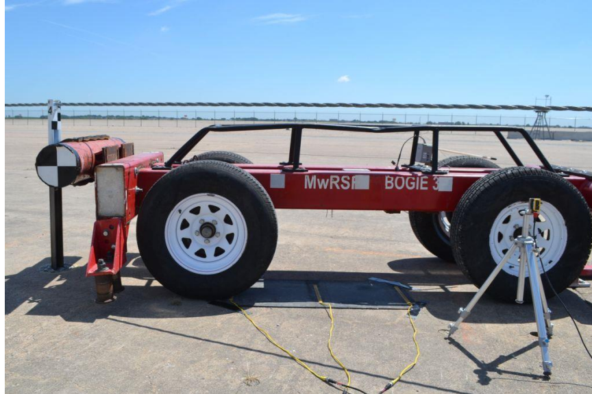
Figure 99. Rigid-Frame Bogie on Guidance Track
