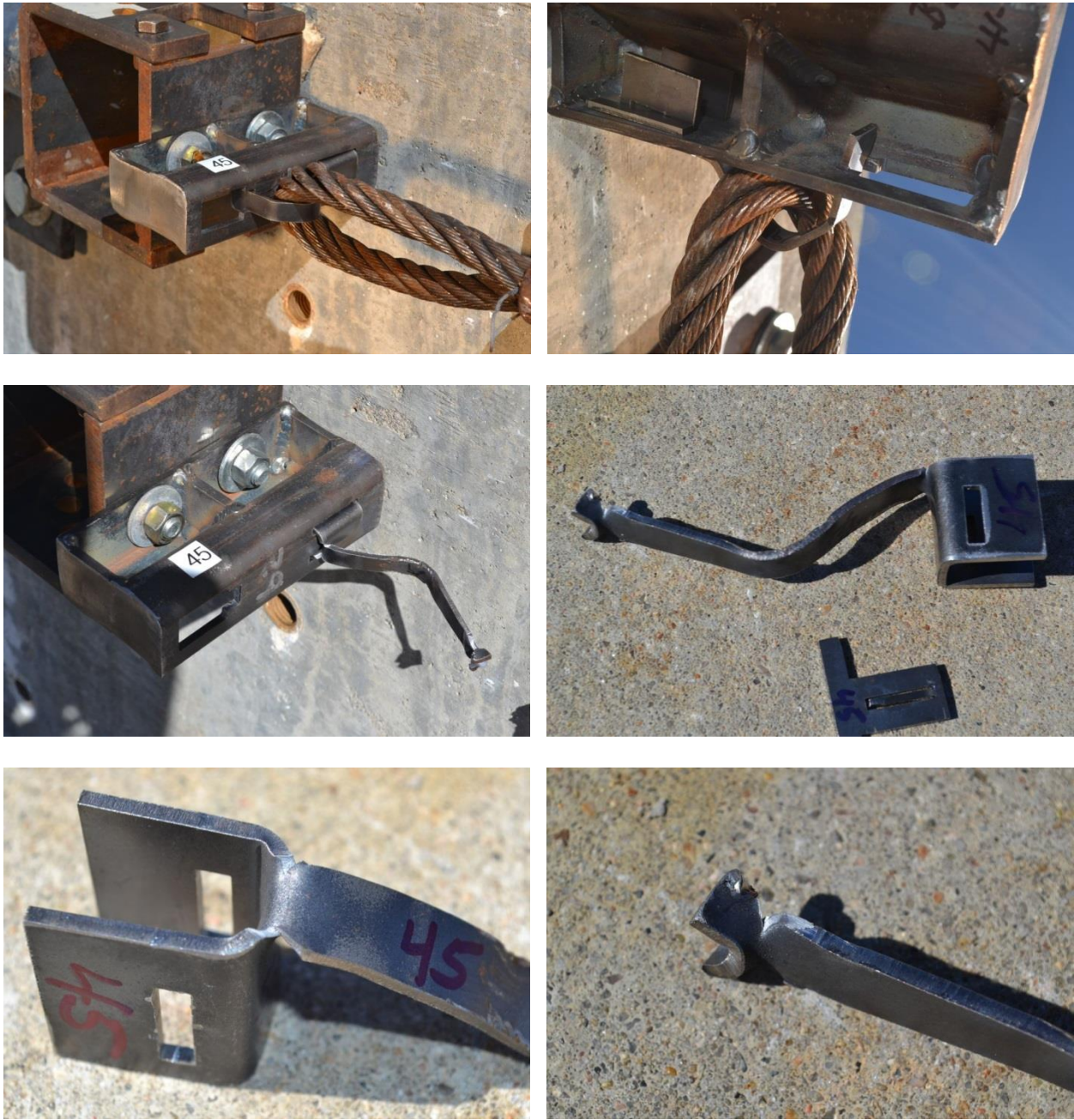
Figure 68. Pre-Test (Upper) and Post-Test (Lower) Photographs, Test No. HTTB-45
