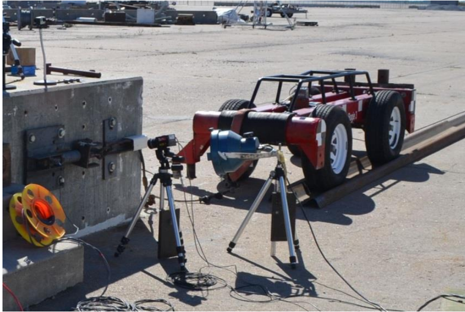
Figure 53. Rigid-Frame Bogie on Guidance Track
