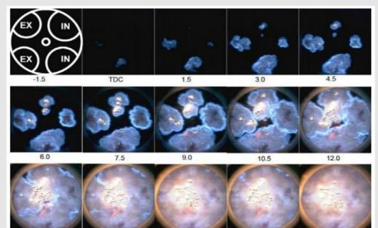
III. Dual fuel combustion – flame propagation – prediction of flame extinction
