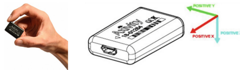
Fig. 1. Axivity AX3 ( 23 \times 32.5 \times 8.9 mm) (left) and axis alignment (right) © www.axivity.com
