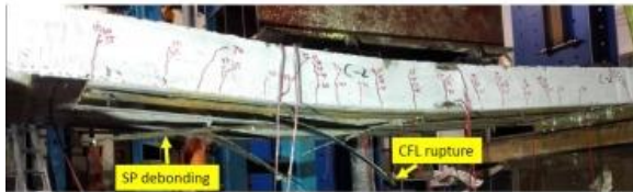
(c) Typical failure mode of Group C
