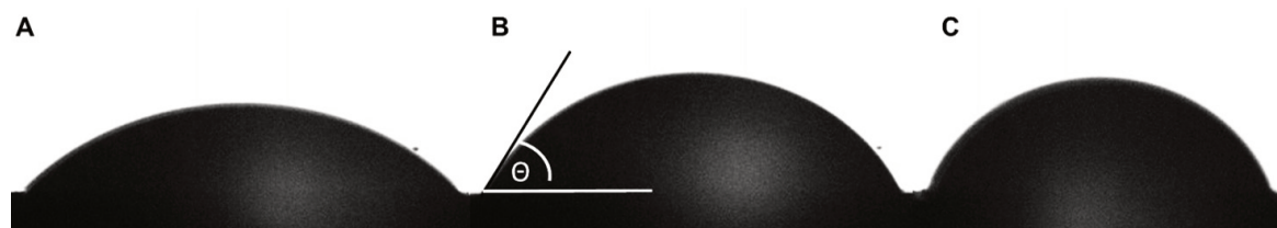
Fig. 3.1: Contact angle between distilled water (20 °C) and alginate (A), xanthan gum (B) and guar gum (C).
