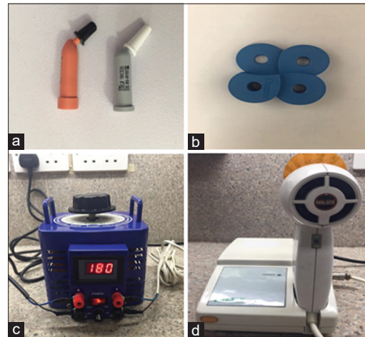
Figure 2: Armamentarium of the experiment. (a) Capsules of the Filtek bulk-fill and SDR restorative material. (b) Plastic molds for packing composites (2, 4, 6, 8 mm depth). (c) Voltage converter. (d) Quartz-Tungsten-Halogen curing light
