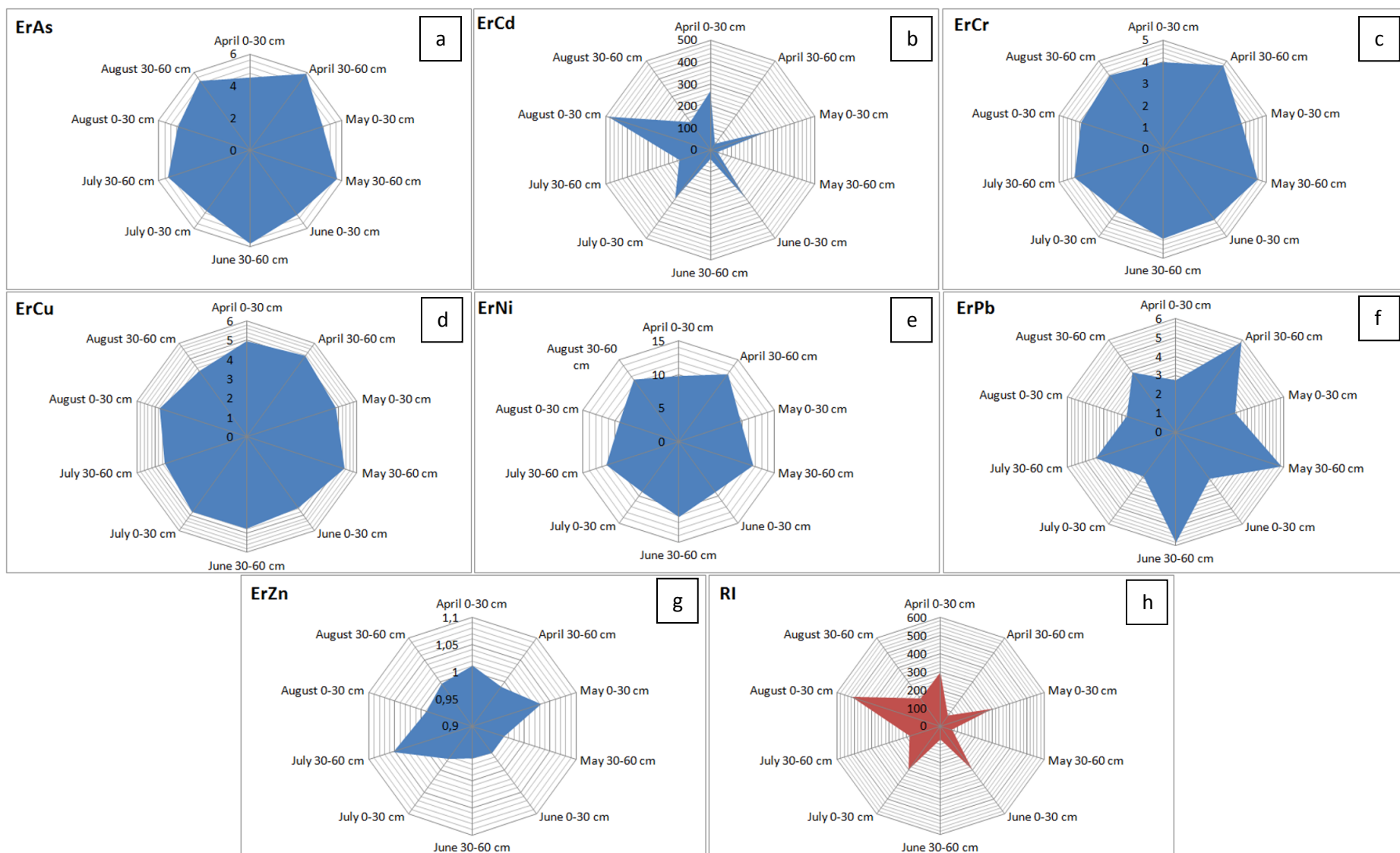
Figure S3. Environmental risk values (-) distribution through the season calculated for both soil layers for a) As; b) Cd; c) Cr; d) Cu; e) Ni; f) Pb; g) Zn and h) environmental risk (RI) (-) for the vineyard soil distribution through the season
