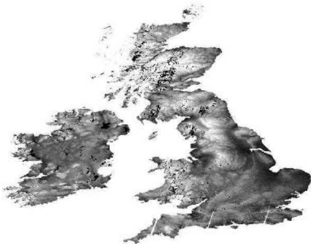
Figure 5 First-Pass IfSAR DEM of the British Isles from the LANDMAP project.
