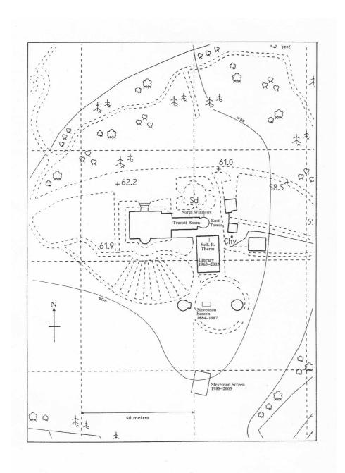
Figure 1: Plan of Armagh Observatory grounds, circa 2000 AD, showing the locations of thermometers used in this study. The East Tower was built in 1827 and the Library in 1963. The north wall screen of the Self-Recording Thermograph was located close to the north wall of the current Library
