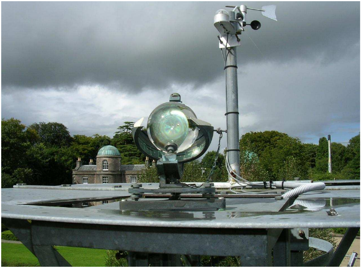
Plate 2. The Campbell-Stokes Sunshine Recorder (centre) with the automatic sunshine recorder and anemometer above and to the right (photo - CJB, Aug 2005)
