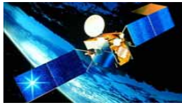
Artist's impression of STENTOR. The propagation package will consist of two beacons, one at 20.7 GHz and the other at 41.4 GHz. It will be launched into a geostationary orbit at 11°W. Both beacons will transmit Right Hand Circular Polarisation signals.
