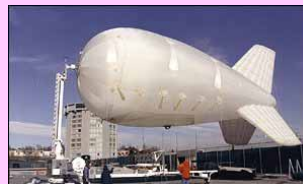
A typical tethered balloon attached to its mast (manufactured by Cameron Balloons Ltd.)
