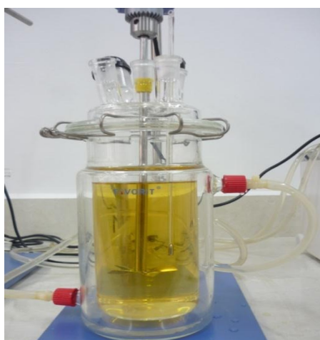
Figure 2: Experimental setup of esterification and transesterification process.
