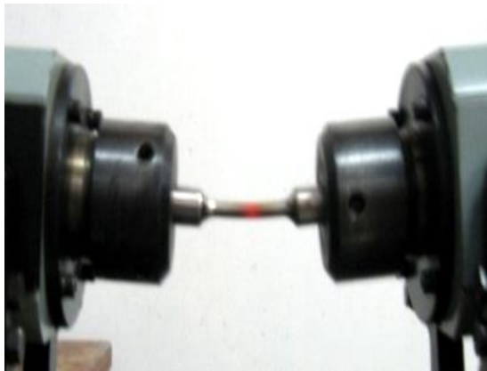
Figure 6. Visual temperature increase for test area of AISI 304 stainless steel at stress 369.53 MPa
