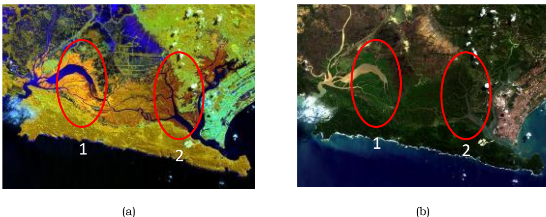
Figure 3-2: Comparison of RGB composites, (a) RGB 564 (False Colour), (b) RGB 432 (Natural Colour).
