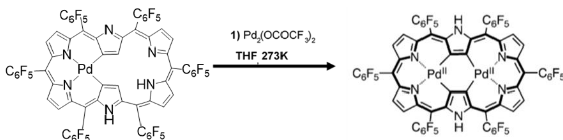
FIGURE 4.4 - Reaction scheme for the synthesis of Pd-Pd [26] hexaphyrin, adapted from reference 176.
