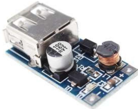
Gambar 9. DC-DC Converter tipe CE8301A
