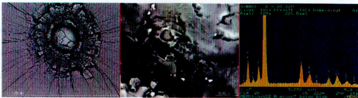
Figure 4.3 BEI of an impact crater produced by shot 22. The second image shows a zoomed in section of the crater seen in the first image. It is clearly possible to see a vesicular residue located on the melt surface most likely produced by shot 22. The ED spectrum obtained for the residue identified enrichments in Na, Mg, Ca and Si (highlighted by the dotted lines) and would therefore be suggestive of a silicate origin.
