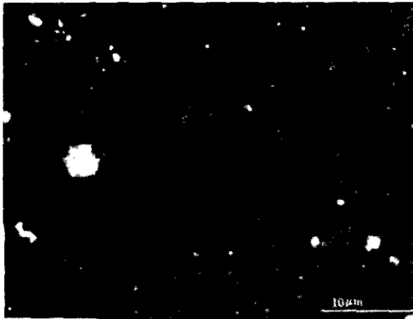
Fig.10 A BEI of Ca-rich fragments retained in the spall zone of a impact crater generated by the calcium carbonate LGG shot. The fragments are comparable to those observed LEO impact craters (Fig.9b).
