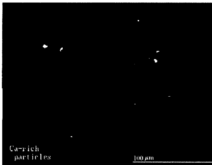
Figure 5.12 BEI of an impact crater generated in LEO, which contains Ca-rich particles in the spall zone. The lack of the particles in the surrounding area would suggest that they are not simply contamination products.
