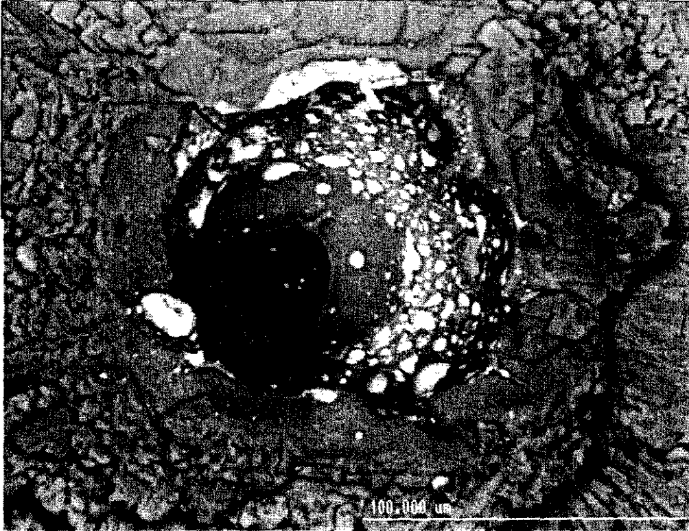
Figure 4.10 BE image of the melt bubble, frozen before collapse. The crater was generated by the pyrrhotite shot and the residue material clearly seen deposited on the surface of the thin bubble layer.
