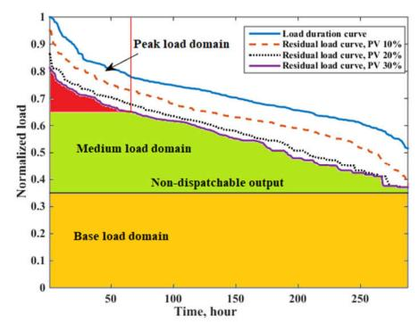
Fig.4-19. Shifted grid load duration curves for different PV capacity integration with dispatch of PHS, twelve representative days, pumping capacity of dispatch PHS to grid peak load ratio is
