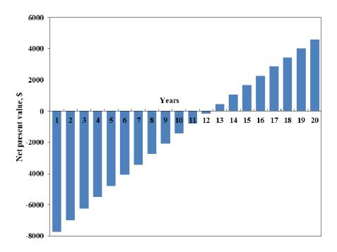
Fig.5-32. Net present value of typical residential PV-battery system, PV 5.0 kWp, battery capacity with 3.0 kWh
