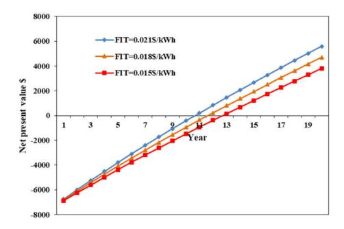
Fig.6-9. Net present value of residential 5 kWp PV and 3 kWh battery system, battery cost 400\$/kWh
