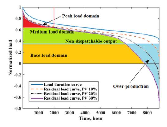
Fig.4-15. Residual load duration curves for different integrated PV capacities based on hourly Kyushu grid load and real PV production during 2016.04~2017.03
