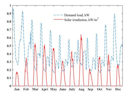
Fig.5-24. Profiles of the residential electricity load and solar irradiation
