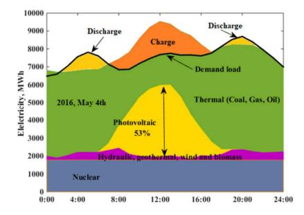
Fig.4-5. Structure layout of the power supply and demand system in Kyushu
