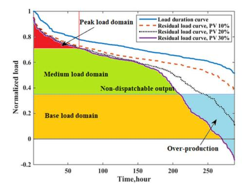
Fig.4-17. Approximation of load duration curve, resulting from daily average load and production profile in months
