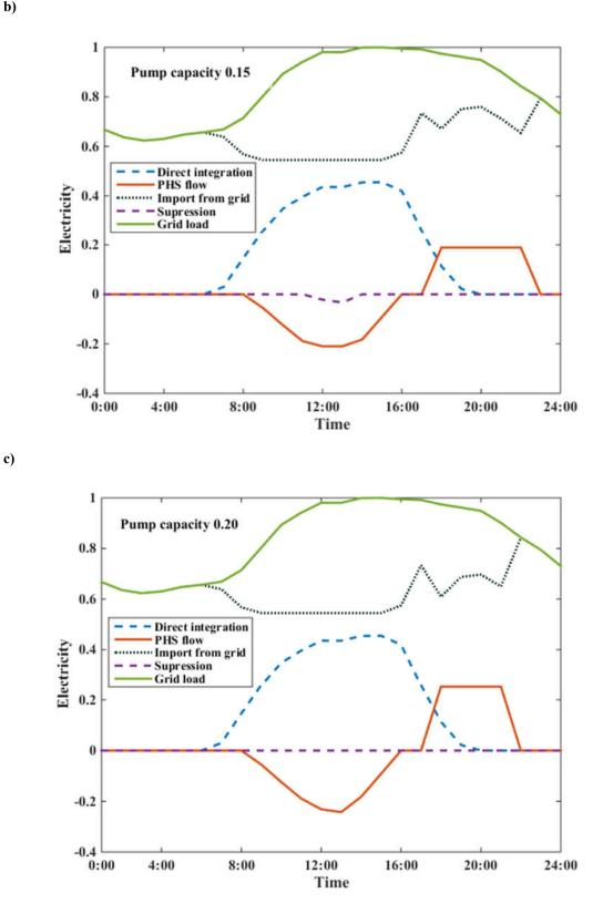
Fig.4-24. Daily power balancing flows in August for different integrated PV capacity (a-c), PV production to grid load ratio at 20%, pumping capacity to grid peak load ratio at 0.10 (a), 0.15 (b) and 0.20 (c)
