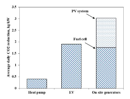
Fig.6-11. Comparison of various high efficiency technologies for average daily CO2 reduction
