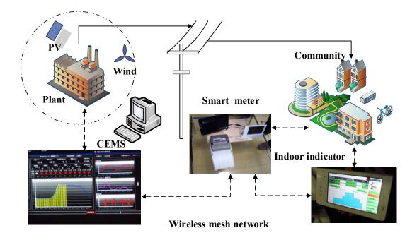
Fig.6-1. Overall structure of the Kitakyushu smart community network
