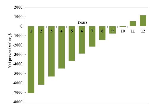
Fig.5-15. Net present value of heat pump water heater system
