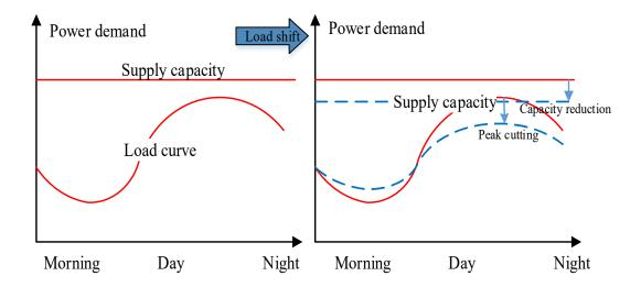
Fig.2-1. Grid load leveling scheme via valley up and peak shave approach
