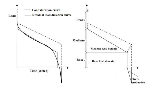
Fig.2-7. The RLDC is a approximated by a box and a triangle, four parts build the sorted load composed of peak, medium, base and over-production parts
