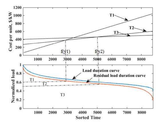
Fig.2-9. Typical screening curve method to analyze optimal generation mix
