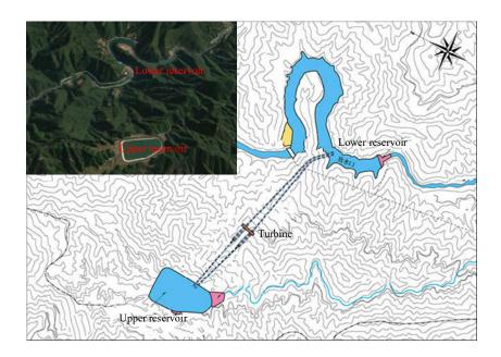
Fig.2-5. The layout of pump storage station in Omarugawa Disctrict, Kyushu
