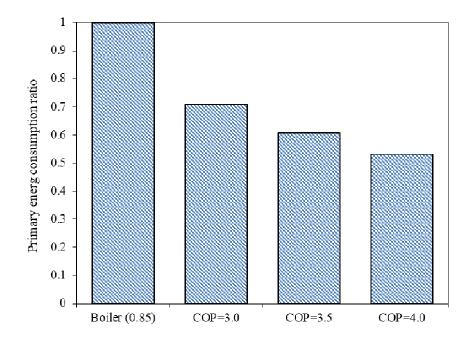
Fig.5-5. Primary energy consumption ratio of conventional thermal boiler and heat pump
