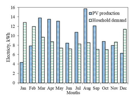
Fig.5-28. Average daily PV generation (5.0 kW<sub>p</sub> capacity) and household electricity consumption of each month
