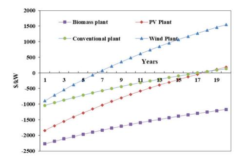
Fig.3-7. NPV of capacity individual plant in 20 years
