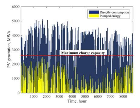
Fig.4-10 Hourly pumped solar energy and directly PV consumption
