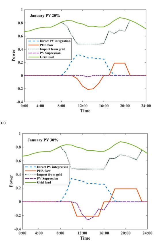
Fig.4-21. Daily power balancing flows in January for different integrated PV capacity (a-c), PV production to grid load ratio ranges from 10%~30%, pumping capacity to grid peak load ratio is
