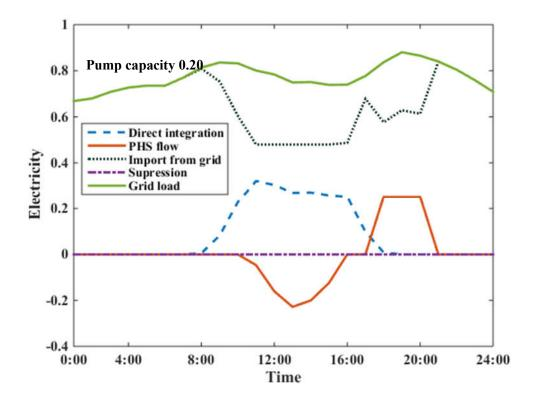
Fig.4-23. Daily power balancing flows in January for different integrated PV capacity (a-c), PV production to grid load ratio at 20%, pumping capacity to grid peak load ratio at 0.10 (a), 0.15 (b) and 0.20 (c)
