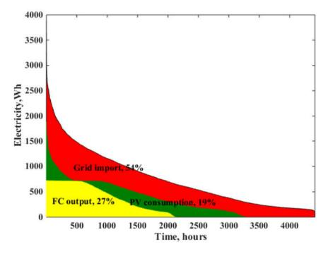
Fig.5-37. Sorted duration curves of fuel cell output, directly PV consumption and demand load
