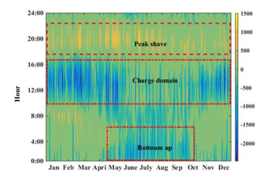
Fig.4-9. Color scale distribution of pumped hydro station
