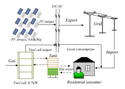
Fig.5-34. Structure of the household hybrid PV/fuel cell energy system
