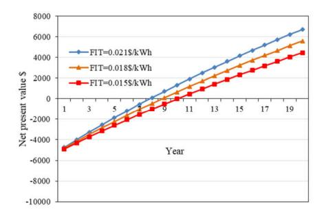
Fig.5-31. Net present values of PV system under different feed in tariffs, PV 5.0 kW<sub>p</sub> capacity without battery
