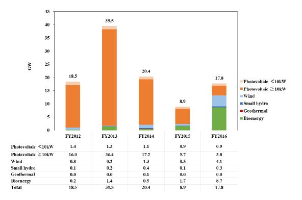
Fig.1-16. Registered renewable energy capacity under FiT in Japan, reference: REI, ANRE/METI Renewable Power Plant Certification Status
