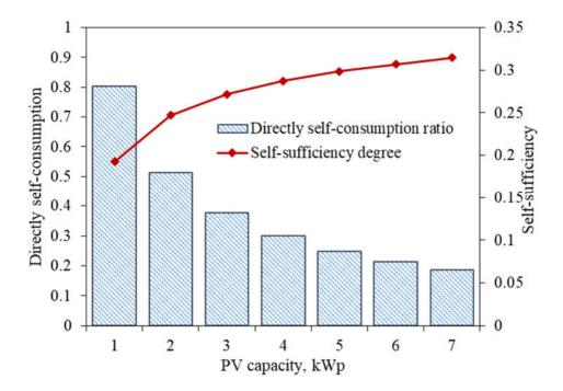
Fig.5-26. Self-consumption and self-sufficiency rates for residential household as a function of the 5.0 kWp PV size, without battery storage system
