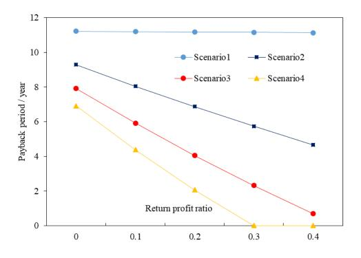
Fig.3-16. The payback periods of VPP under different return profit ratio from plant side
