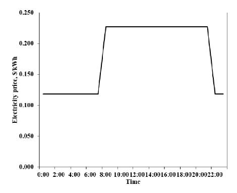
Fig.5-14. Time of use tariff structure, reference: Kyuden Power Company
