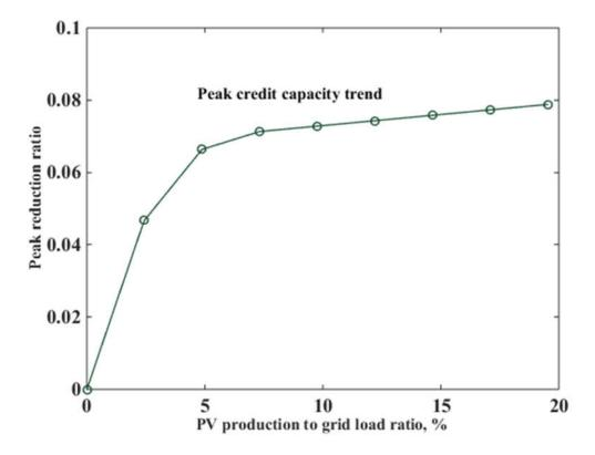
Fig.4-14. Peak reduction ratio as function of PV production to grid load ratio
