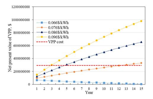
Fig.3-14. NPV of power plant side under different electricity feed-in tariffs
