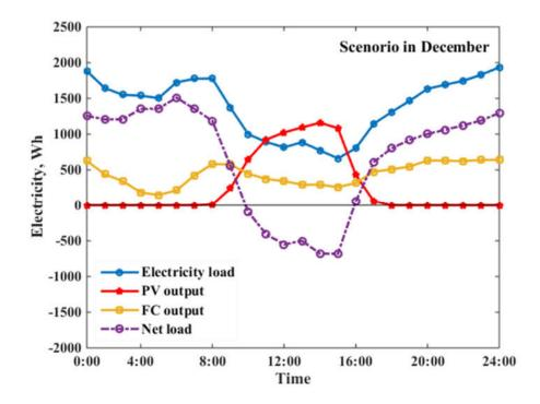
Fig.5-41. Daily power matching scenarios of the grid-tied Net ZEH: average hourly electricity load, PV output, FC generation and net load profiles in August (a), October (b) and December (c)
