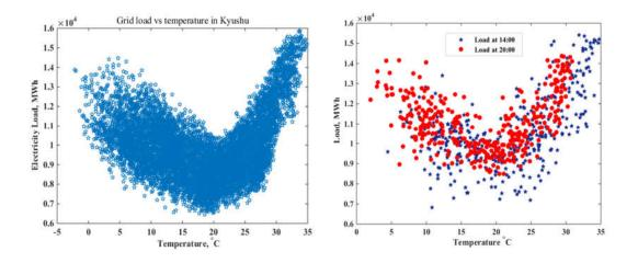
Fig.4-12. The temperature sensitivity of peak load in Kyushu
