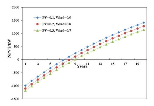
Fig.3-8. NPV of capital combined PV and wind turbine power plant
