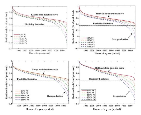
Fig.2-8. Residual load duration curves for different integrated PV capacities based on Kyushu, Shikoku, Tokyo and Hokkaido, grid loads and real PV productions in period of 2016.04~2017.03
