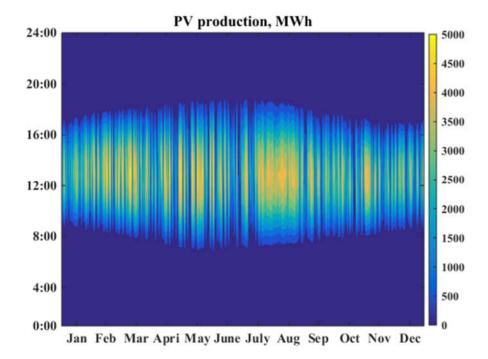
Fig.4-8. Color scale distributions of solar PV production in Kyushu
