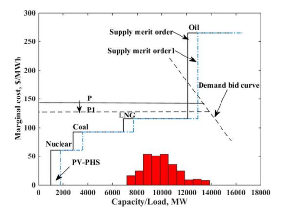
Fig.4-30. Merit order effect of PV-PHS in Kyushu power supply system
