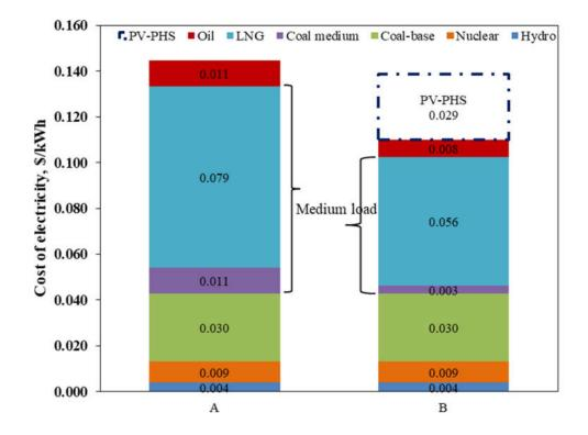
Fig.4-34. Comparison of electricity generation cost between different power mix struture
