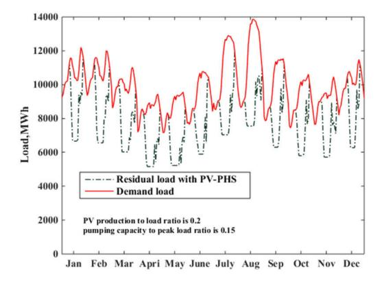
Fig.4-25. Daily demand load and residual load profiles with PV-PHS, PV production to load ratio is 0.2, pumping capacity to peak load ratio is 0.15
