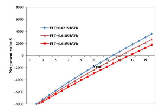
Fig.6-8. Net present value of residential 5 kWp PV and 3 kWh battery system, battery cost 8008/kWh
