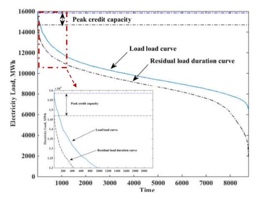
Fig.4-13. Peak credit capacity of PV at PV production to grid load ratio is 9.76%
