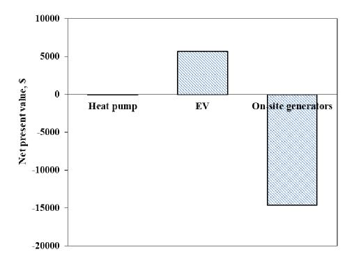
Fig.6-10. Net present value of high efficient technologies within 10 years from 2017 to 2027
