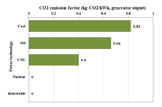
Fig.1-2. Electricity generation carbon emission factor by source, reference: Power Generation Cost Verification Working Group 2015
