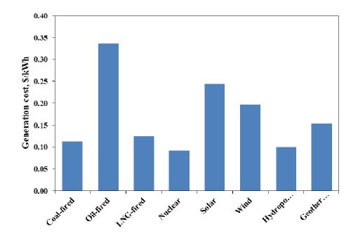
Fig.1-1. Electricity generation cost by source, reference: Power Generation Cost Verification Working Group 2015
