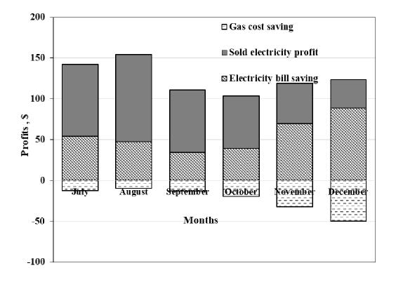
Fig.5-43. Profit components of the ZEH with hybrid energy system (PV system 4.84 kWp, Fuel cell 0.70 kW) from July 2017 to December 2017
