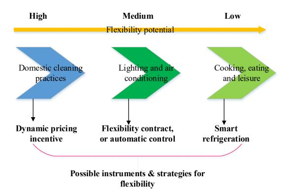
Fig.2-6. Flexibility of electricity appliances in demand side
