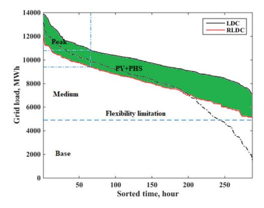
Fig.4-31. Impacts of PV+PHS on load duration curves, dash dot line refers the residual load duration curve without PHS
