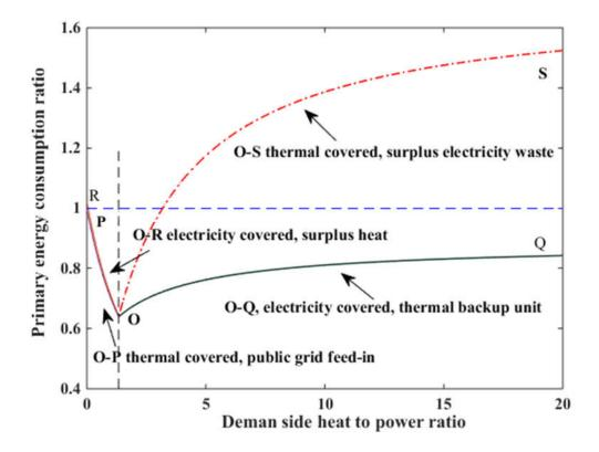
Fig.5-36. Primary energy saving performance of fuel cell cogeneration system
