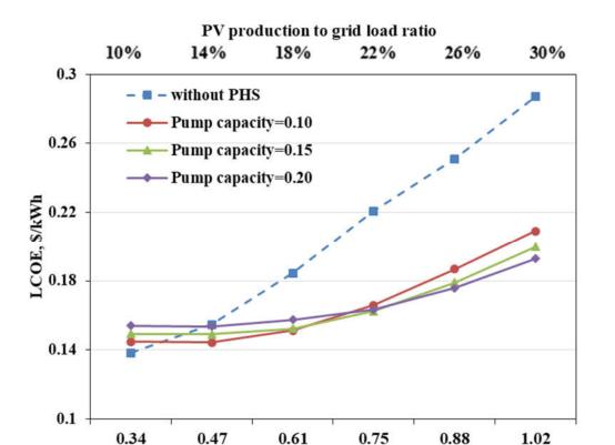
Fig.4-27. The average lifetime levelized cost of electricity generation for PV systems with different integrated pumping capacities of PHS
