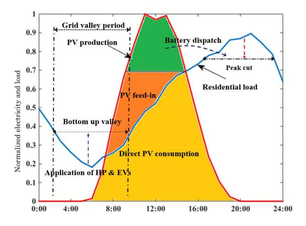
Fig.2-10. Schematic representation of demand side management from bottom up modeling approach
