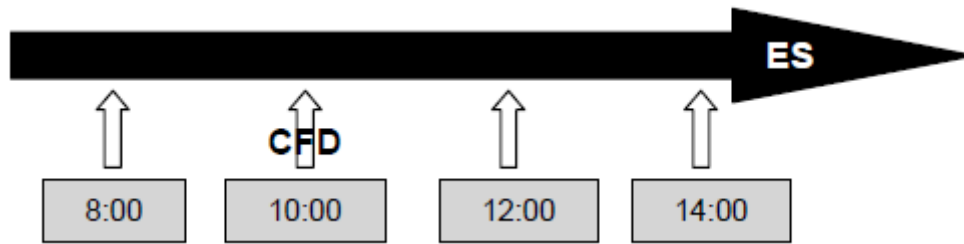
図 2.1.1.4-2 Illustration of time coupling (ES handles a long-term simulation, such as a design day, while CFD runs only at some specific times, such as 8:00 am). 文4)
