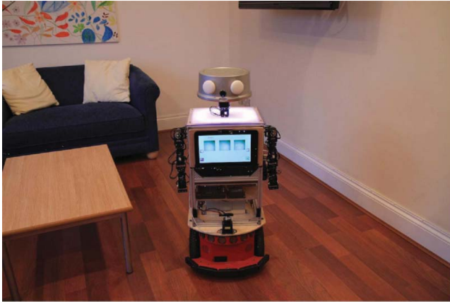
FIG. 4. Interacting with the touch-screen interface on the Sunflower robot.
