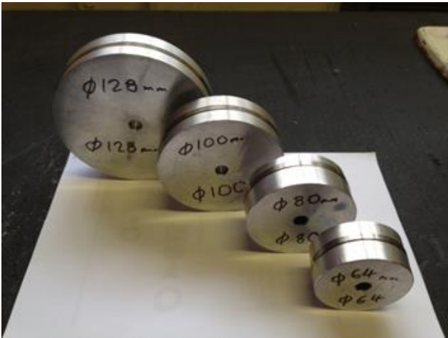
Fig. 5 showing typical roundness formers used
