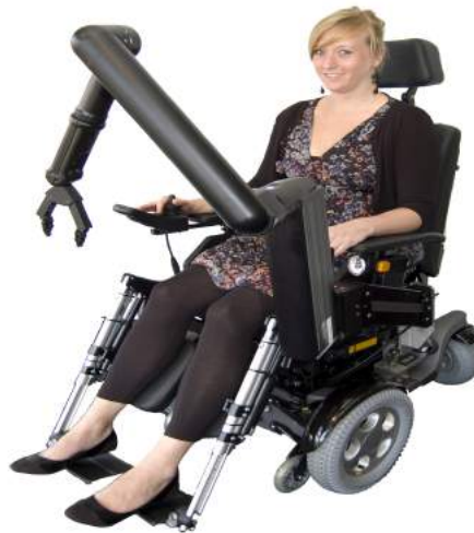
Figure 2.5: iARM (intelligent Assistant Robot Manipulator) Image courtesy Assistive Innovations bv and Exact Dynamics
