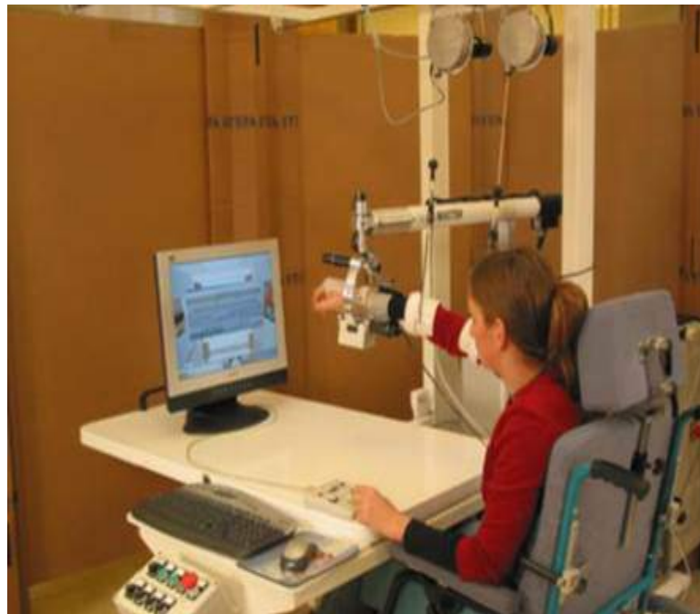
Figure 2.11: GENTLE/S rehabilitation system Image courtesy Prof. William Harwin
