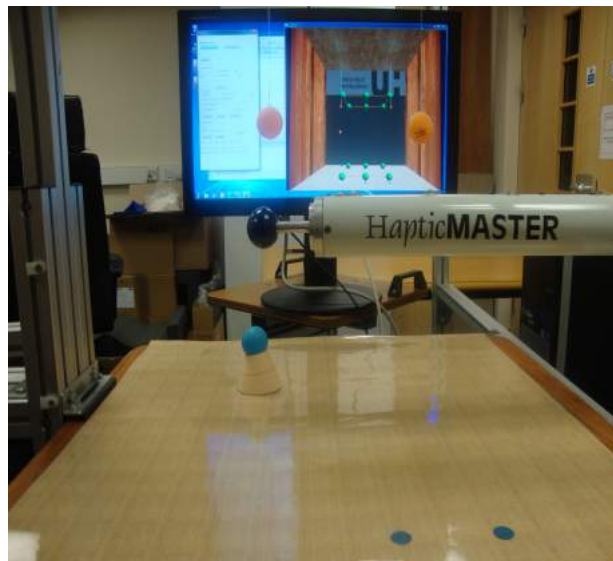
Figure 4.2: Embedded set-up (showing both Virtual targets (on screen) and real targets (Ping-Pong balls and stickers on the table mat))
