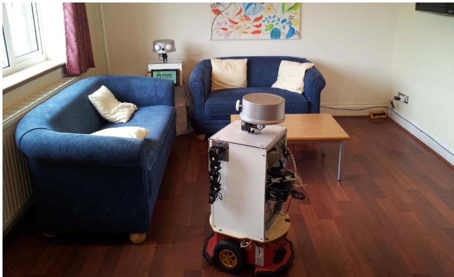
Fig. 1. Robot House Living Room Area. It shows one mobile Sunflower robot in the front, and a stationary Sunflower robot in the back.
