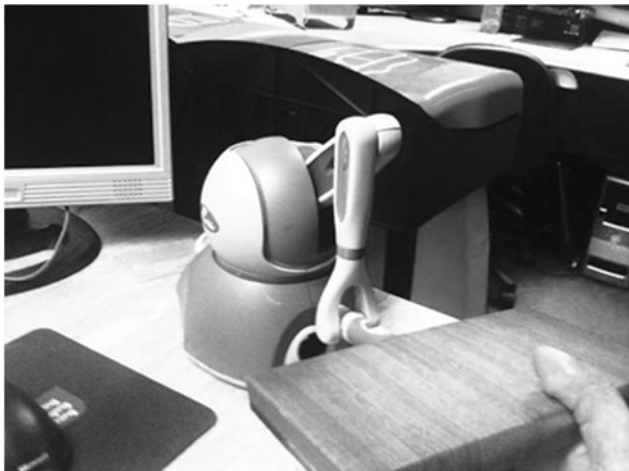
FIG. 2. The Phantom Omni with Styrofoam board extension.
