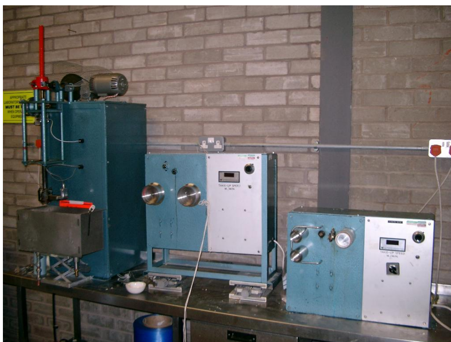
Fig. 3.6 Bradford University Research Ltd. Small Scale Ram Extruder
