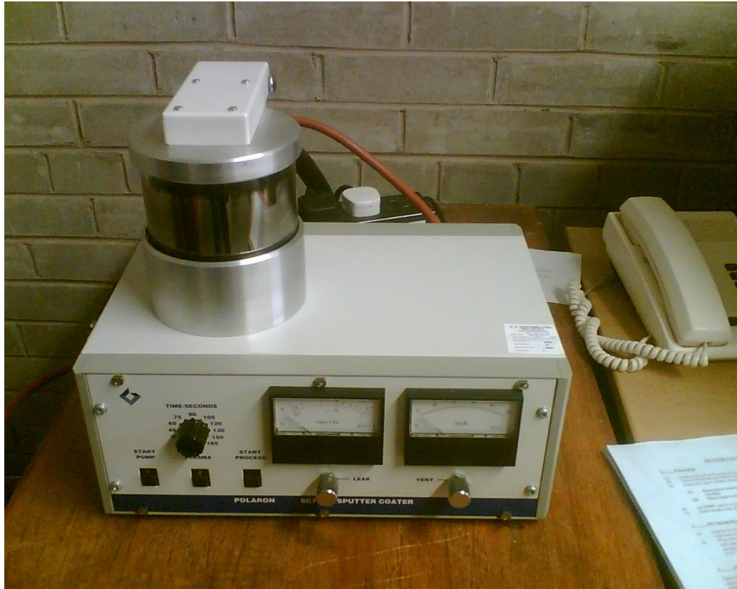
Fig. 3.11 - Polaron sc7620 sputter coater
