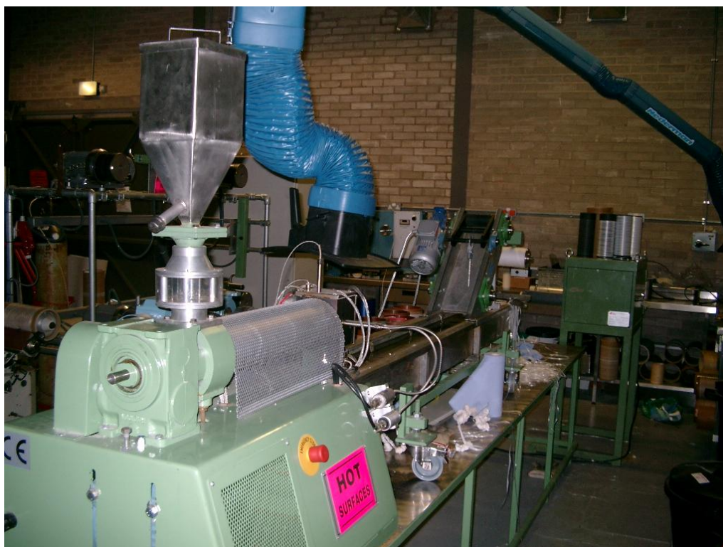
Fig 3.4 ESL Laboratory Extrusion, Melt Spinning and Draw Equipment. Labspin 892.
