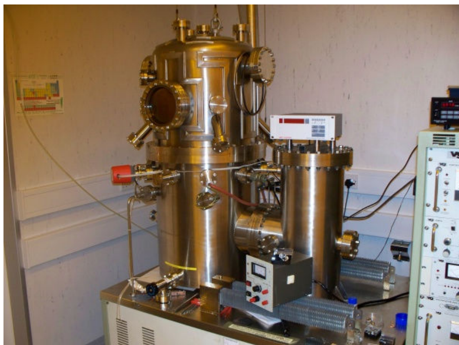
Figure 3.9: High Vacuum Chamber used for growth of amorphous \text{SiO}_2 thin films using electron beam evaporation.
